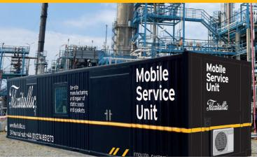
The mobile service unit is provided during shutdown periods to offer additional support for all gasket related issues. The primary purpose is to manufacture and refurbish a wide range of gaskets.
