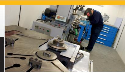
The mobile service unit is well equipped with a range of machines for manufacture and repair/refurbishment of a range of gasket types and styles.
